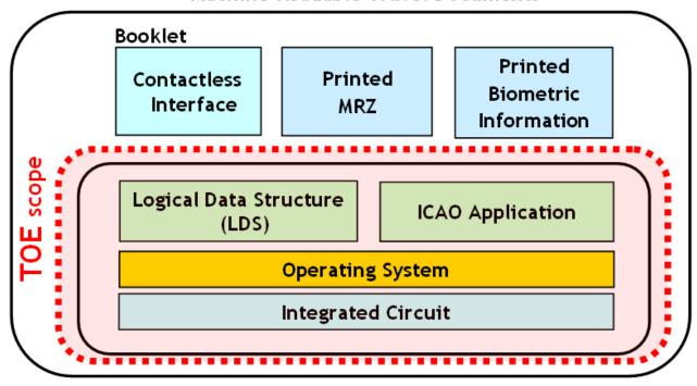
The TOE is defined to comprise the chip and the complete operating system and application. Note, the inlay holding the chip as well as the antenna and the booklet (holding the printed MRZ) are needed to represent a complete MRTD, nevertheless these parts are not inevitable for the secure operation of the TOE.
